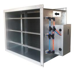
The AFMS is an accurate airflow measuring station and is furnished with a properly sized pressure transducer that outputs a signal proportional to CFM. It is designed to maintain a constant parallel airflow pattern over the static sensing ports for more accurate, steady signals under all duct conditions.
