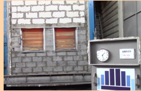
Cosmos Fire Dampers During Fire Endurance test at UL Laboratories
