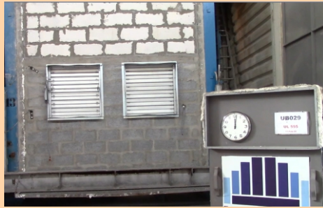
Cosmos Fire Dampers During Fire Endurance test at UL Laboratories
