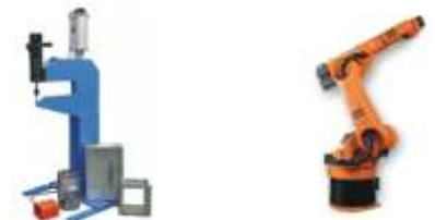
Clinching Machine welding Robot
