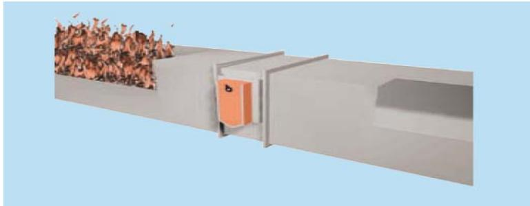
The COSMOS smoke damper prevents the spread of fire and smoke in rectangular ducts. The smoke damper shuts a ductwork branch off in order to prevent the propagation of flue gases in the ventilation system. In the closed position, the airflow leakage through the damper is very limited.
